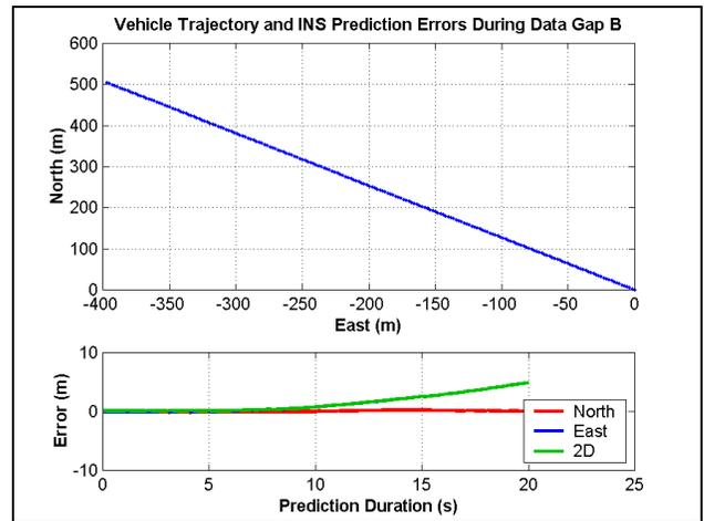
**Figure 7 - Vehicle Trajectory and INS Prediction Errors During Data Gap B**
