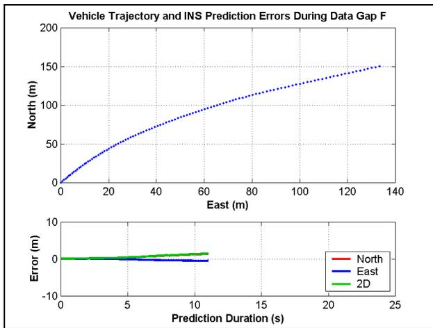
**Figure 11 - Vehicle Trajectory and INS Prediction Errors During Data Gap F**
