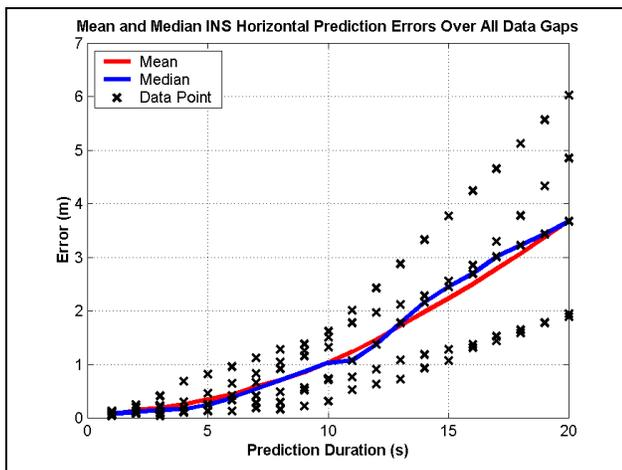
**Figure 12 - Mean and Median INS Horizontal Prediction Errors**
