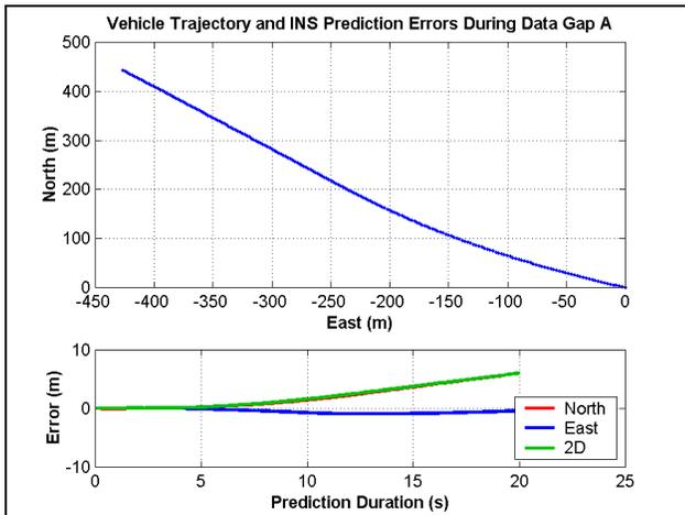
**Figure 6 - Vehicle Trajectory and INS Prediction Errors During Data Gap A**
