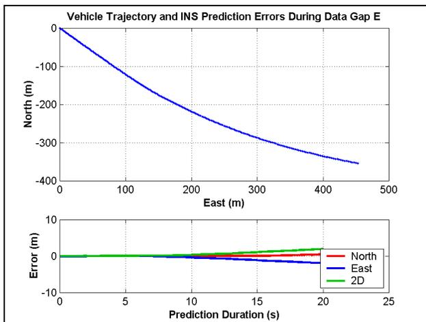
**Figure 10 - Vehicle Trajectory and INS Prediction Errors During Data Gap E**
