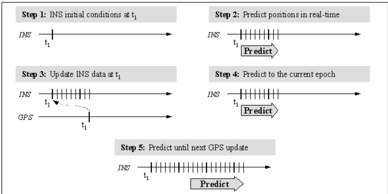
**Figure 1 - Graphical Description of how to Update the INS with Latent GPS Data**
