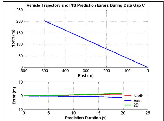
**Figure 8 - Vehicle Trajectory and INS Prediction Errors During Data Gap C**
